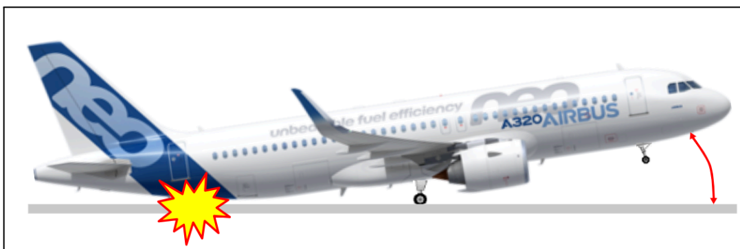
Illustration A-5: V_{MU} Demonstration (Geometrically-limited Aircraft)
